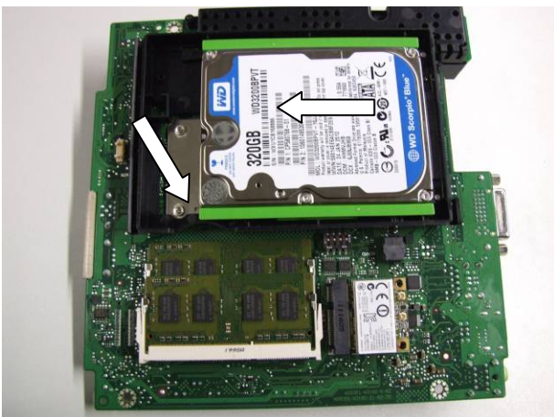
Press the small hard disk carrier downwards and at the same time push the hard disk in the direction indicated by the arrow.
