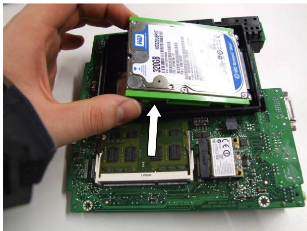
Lift out the hard disk.
